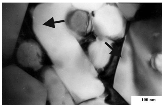
Fig. 10. TEM observation of recrystallised intergranular phase (arrows) in the \text{Si}_3\text{N}_4/\text{SiC} nanocomposite (composition 2).
